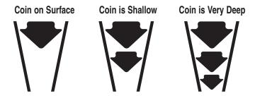
Objects other than coins will still register on the 3-segment depth scale, but the depth indication will be relative. For example, all 3 segments illuminated could indicate a coin buried 9" deep, but could also be a very large object several feet deep. Use the Depth Indicator in conjunction with the Conductivity Arc to gain more information.
